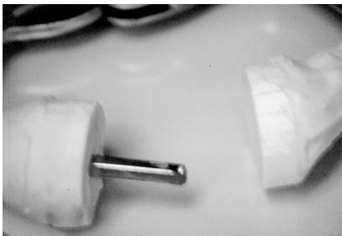
FIG. 2—Trauma induction implement used in the study. Instrument consisted of a modified mechanical vise grip with the tissue sample held in a plastic plate on one jaw, and the aluminum die on the other jaw.
